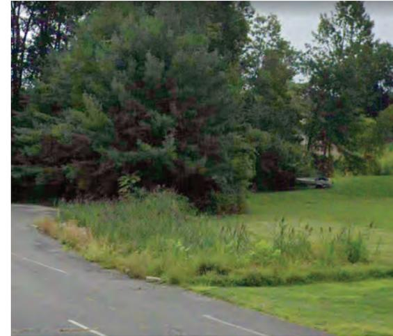
A section of parking spaces can be converted to porous asphalt to capture and infiltrate stormwater runoff from the parking lot. A small detention basin can be retrofitted to a rain garden to create native pollinator habitat and capture, treat, and infiltrate runoff from the parking lot. A preliminary soil assessment suggests that more soil testing would be required before determining the soil's suitability for green infrastructure.
